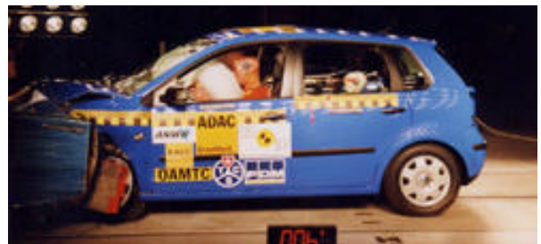
Offset crash test at 64km/h
