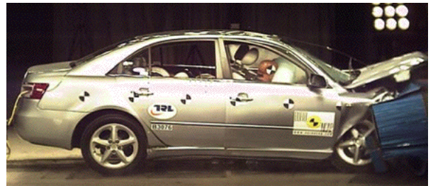
Offset crash test at 64km/h
